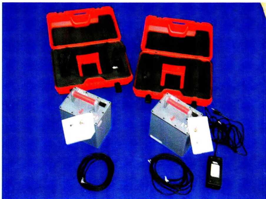
Foto 11. Batery dan Charger Laser Scanner
