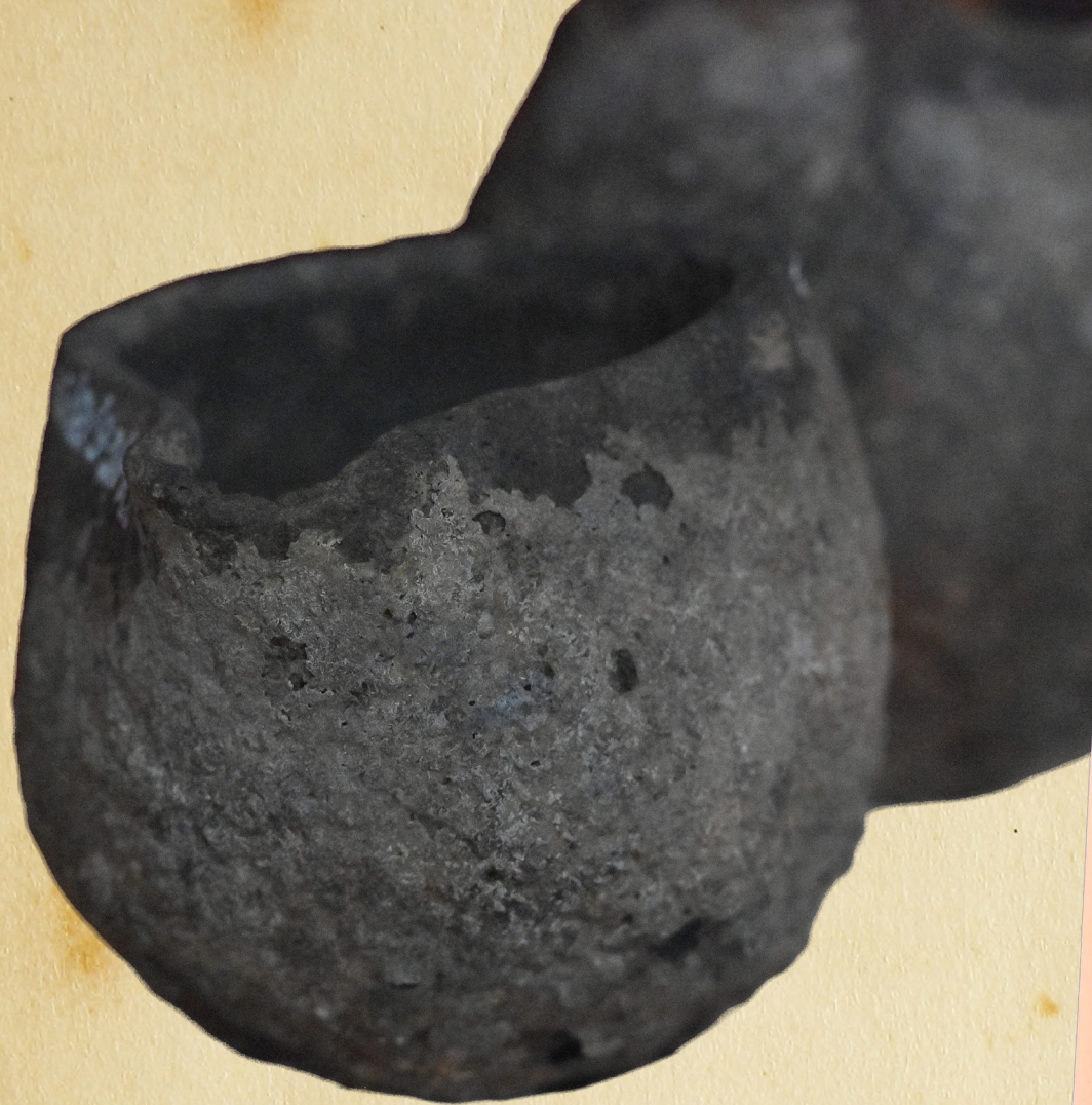
Kowi, a crucible used to melt metal before it is poured into the mold Photo: Syefri Luwis
