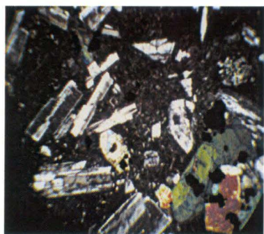
Figure 1. x40; Crossed Nichols. Stone texture showing simply geminated plagioclase crystals and olivine crystals including opaque minerals.
