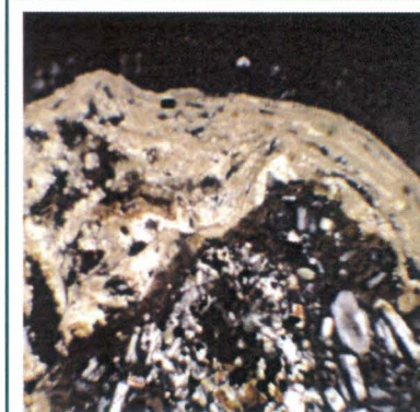
Figure 3. Sample T2J-16a; x100, Nichols +. The crust of calcite is due to several deposition mechanisms.
